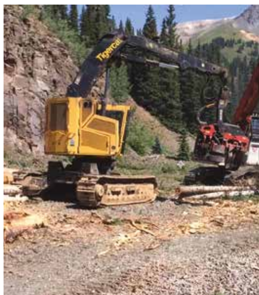
Above Highway 550, a timber loader and a logging processor turn felled trees into lumber.
